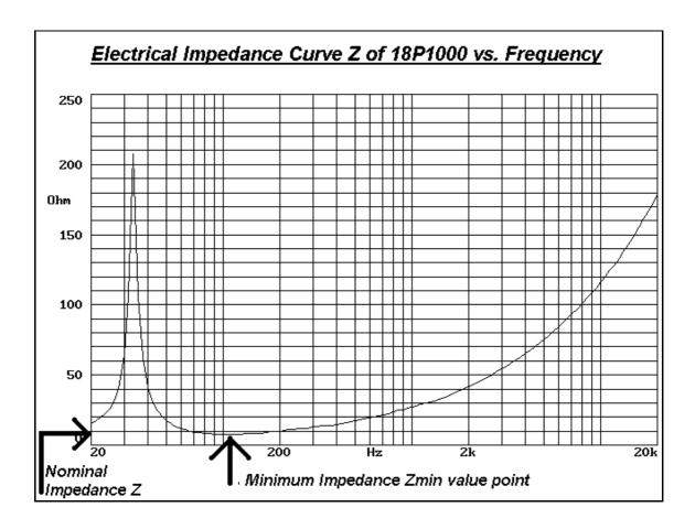
For example, the 18P1000 model, from the **beyma** P1000 series, with 8 ohms nominal impedance has a  $Z_{\text{min}}$  value of 7,4 ohms at 120 Hz. For that reason, in RMS value, a power of 1000 watts would come given by an applied tension of 89 Volts RMS. However, in AES power, this value would be of 86 Volts RMS.
